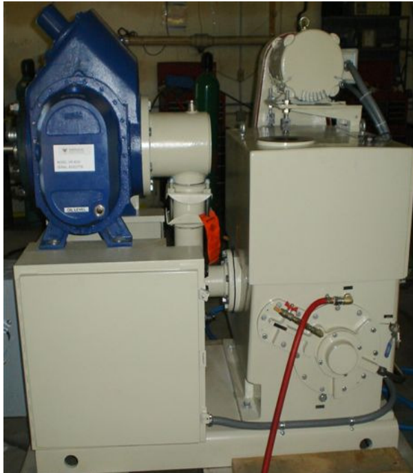
1722 STYLE PUMPING SYSTEM WITH BY-PASS BLOWER
